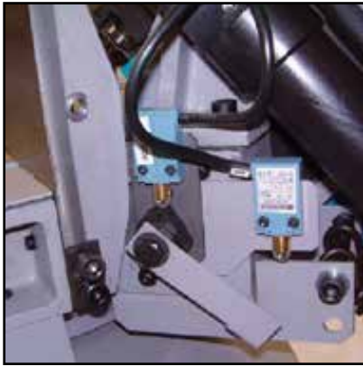
Device to synchronize the RTD/RTP table and the head motion Device to synchronize the RTD/RTP table and the head motion
