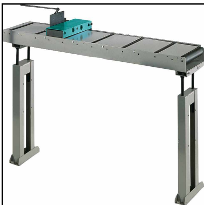
Unloading roller table with metric rod and length stop (Optional) OPTIONAL
