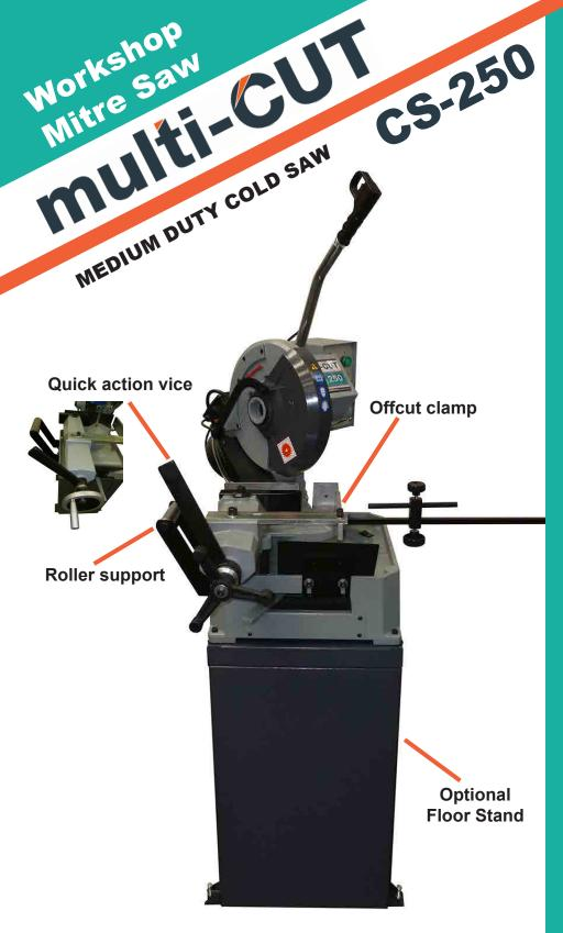
Recommended for the busy workshop, this modern well proven machine offers both precision and reliability. Loaded with standard high quality features it represents unbeatable value.
