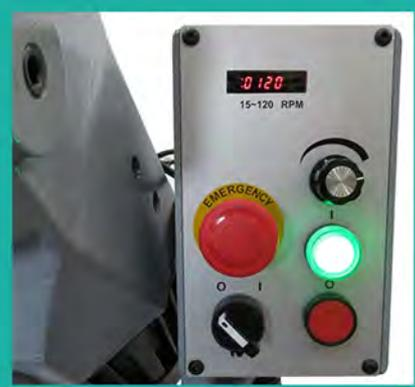
Variable blade speed with inverter 15~120rpm
